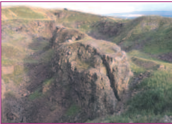
Photo 43. West Rigg Opencut, Westgate, Weardale. Worked out iron ore flats adjoining Slitt Vein. The vein remains as an unworked pillar in the centre of the quarry.
