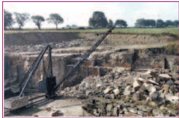
Photo 77. Dun House Quarry, Stainton. Namurian sandstone worked as building stone.
