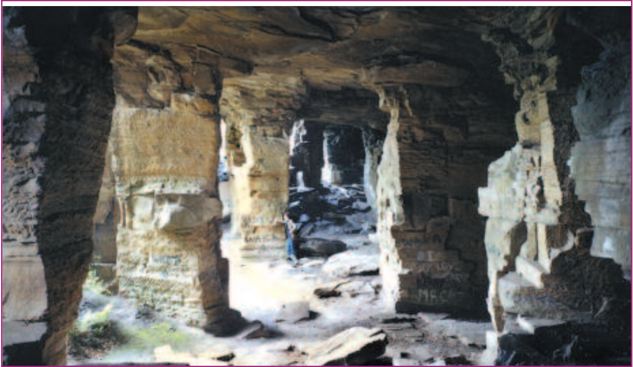
Photo 19. Hown's Quarry, Consett. Underground quarries in the sandstone between the Marshall Green and Victoria coals.
