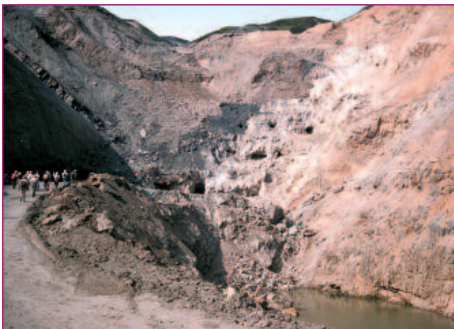
Photo 41. Closehouse Mine, Lunedale. The wide barytes vein adjacent to the Lunedale Fault. Photographed 1984.
